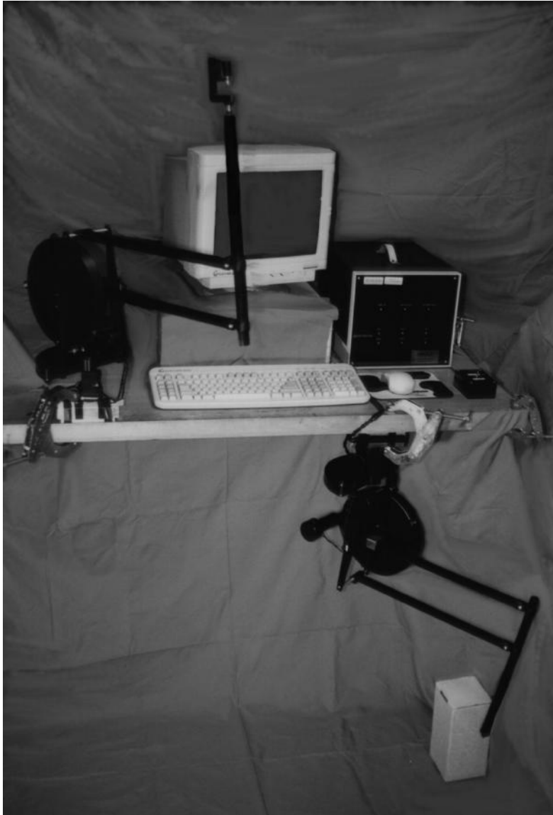
Figure 1-3: The experiments are performed using two robots with three degrees of freedom each. The master is shown on the left reaching up, while the slave is on the right interacting with objects on the floor. The controllers match their cartesian tip motion, so that the user may ignore the kinematics.
