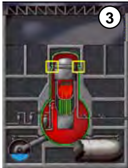
Containment pressurizes. Likely leakage at drywell
