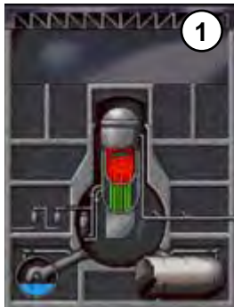
Core damaged but retained in vessel
