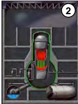
Some portions of core melt into lower RPV head
