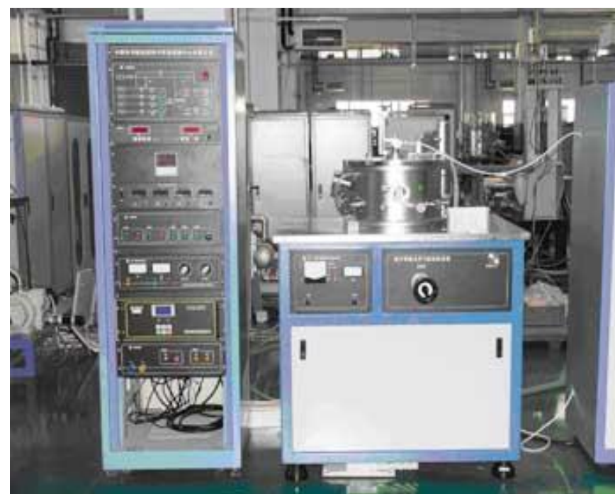
等离子增强化学气 相沉积系统 Plasma enhanced chemical vapor deposition system
