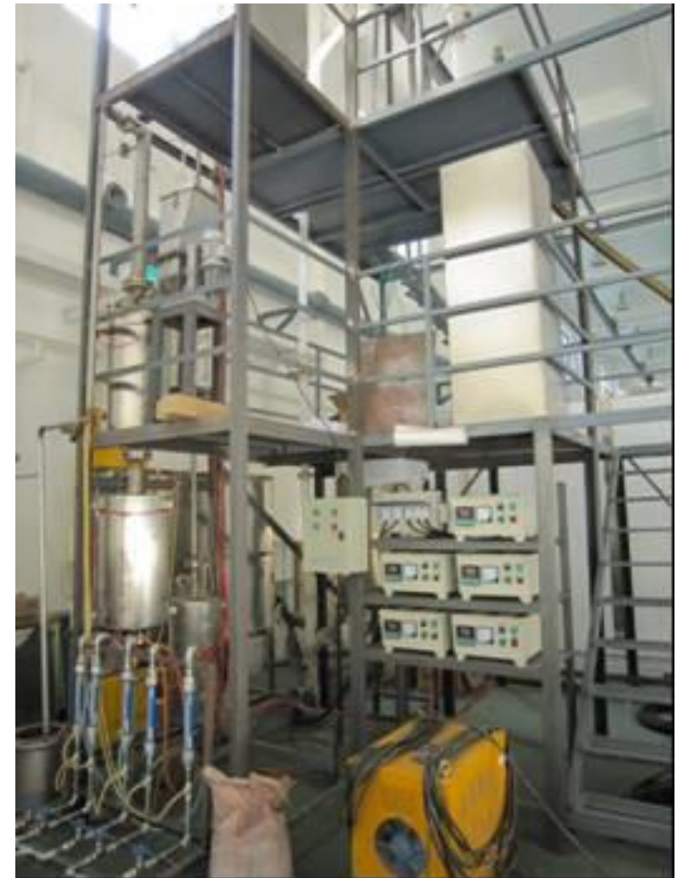
生物质气化试验平台 Experimental Platform for Biomass Gasification
